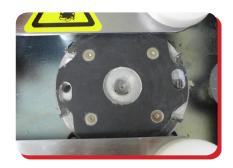
New spine roughening with 1 notching blade and 6 roughing blades provides better glue penetration while applying the glue onto the book spine.
